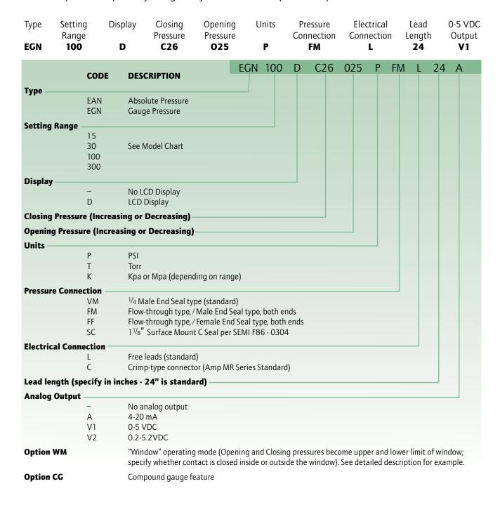
The specified example denotes a 100 psig Staset® switch with LCD display. The switch closes on increasing pressure at 26 psig and opens on decreasing pressure at 25 psig. The switch utilizes a flow through design with  $\frac{1}{4}$  male end seal type end connections with a 5 Ra finish. The electrical interface consists of 24" free leads. A 0-5VDC analog output is provided.
